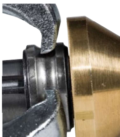
Lock on ball grooves and bearing races.
