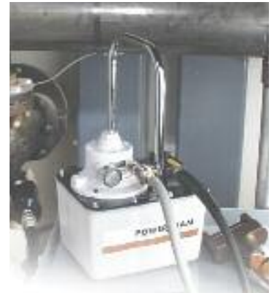
The PA17 used with a flange spreader
